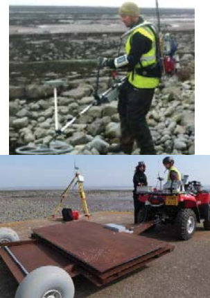
Figure 2. Cefas’ sweeper (left) and swath (right) RFID detector and positioning systems
