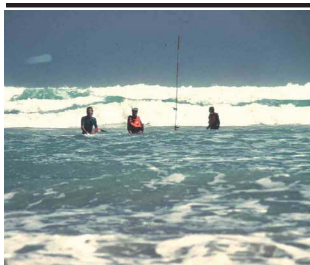
Figure 2. Deploying field equipment in the dissipative Goolwa surf zone, 1980. The aerial holds pressure sensors and current meters and indicates location in deeper water.
