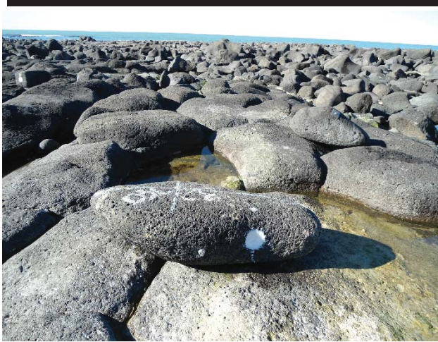
Figure 6. The first movement of boulder L3. The boulder was rolled on 4 April, 2013 when wave height was recorded as Hsig 0.64 m.
