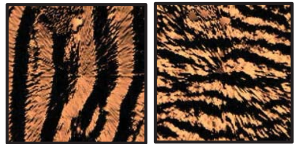
Figure 2. Example of wave ripple, W, (left panel) and current ripple, C, found off South-Holland coast.
