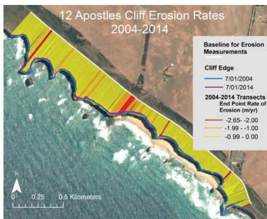
Figure 8. Erosion rates of the modern limestone cliffs from 2004 - 2014.
