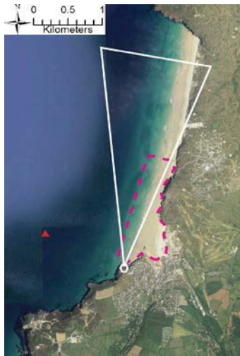
Figure 1. Satellite image of Perranporth beach. The octagon and open triangle show the location and field of view of the Argus cameras, the dashed line shows the typical extents of the topographic surveys, and the solid triangle shows the location of the nearshore wave buoy.
