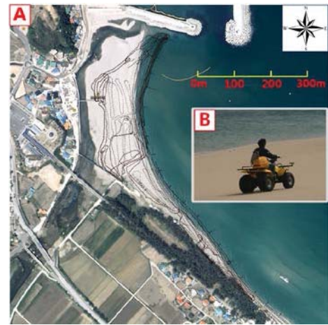
Figure 8. (A) Point data of continuous measurement using RAS method, and (B) RTK-GPS system mounted on an ATV.
