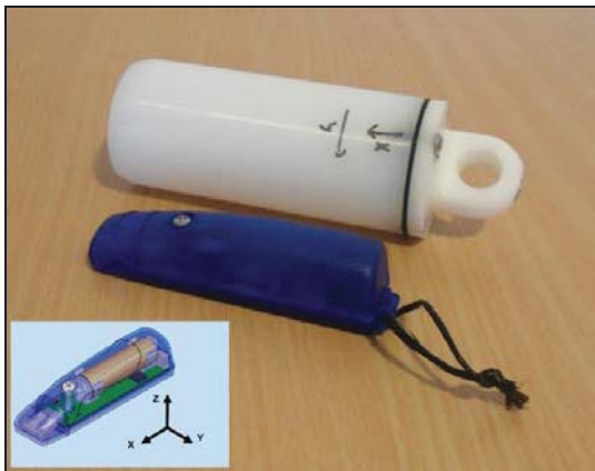
Figure 3. Waterproof housing and a GCDC accelerometer (100×25×25 mm) used to record boulder movements (Photo: Alenka Abazović. Insert: GCDC, LLC).
