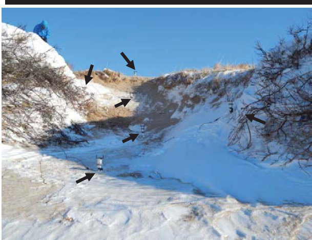
Figure 5. A trough blowout at Cape Cod. The blowout was formed as a discrete saucer blowout and evolved into a trough blowout as the adjacent erosional ridge was notched. The flow experiment was conducted in this blowout. The arrows indicate the position of the sonics. The most distant sonic anemometer (no. 4) is on the depositional lobe.
