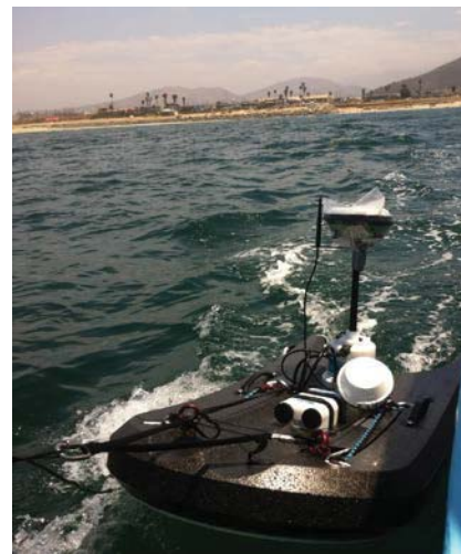
Figure 2. ADCP and differential GPS mounted on the hydroboard and towed on the side of the surveying boat. An example of set-up during the measurement collection.
