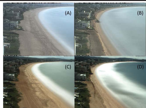
Figure 2. Pre- and post-storm images (looking north) taken from the Narrabeen-Collaroy ARGUS video monitoring station for: (A-B) the June 2007 ECL; and (C-D) the April 2015 ECL. All images are 10-minute time exposures taken at mid tide.
