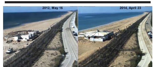
Figure 5. Oblique images of camera 6 showing the disappearance of the beach and shoreline 3D pattern after the adaptation period following the deployment of the submerged structure.
