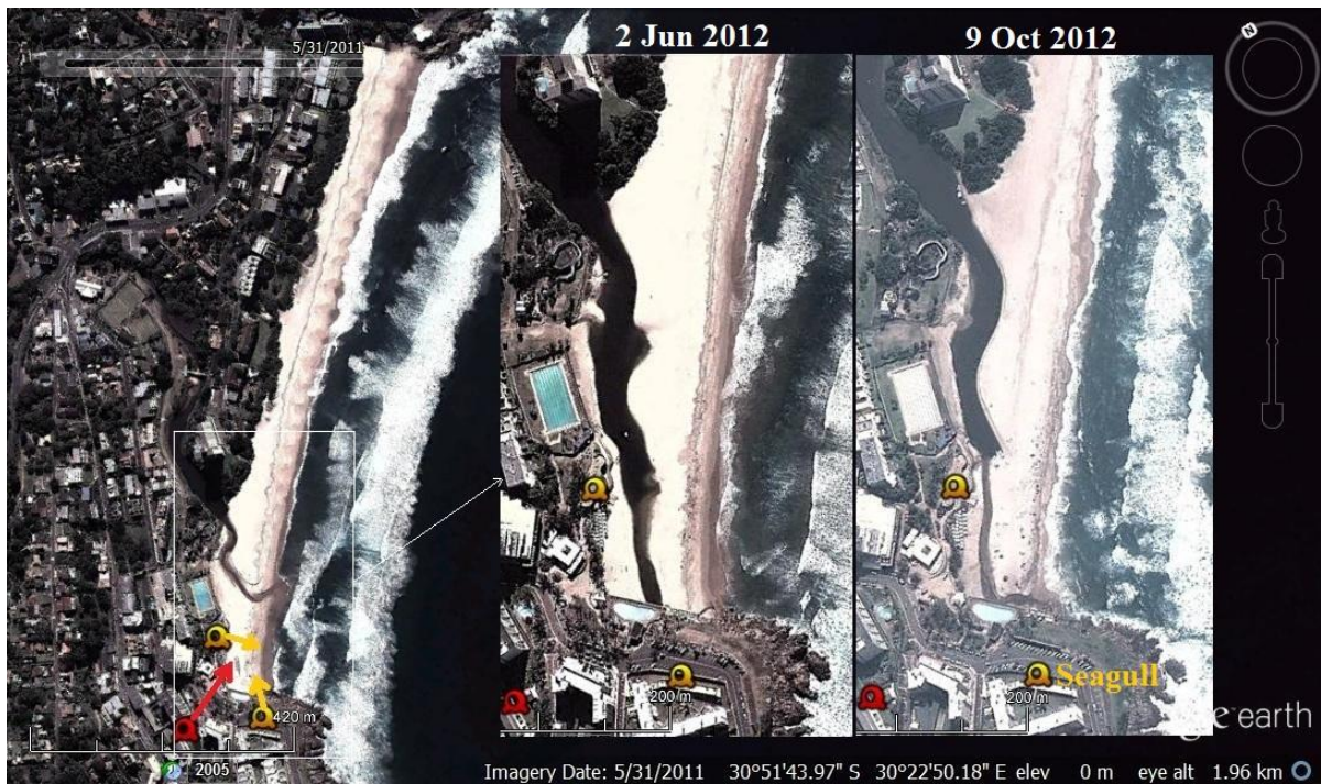
Figure 2. Google Earth imagery of Margate beach showing Nkongweni lagoon mouth position on 31 May 2011 and location of webcams in the south. The Vodacom webcam locality and view direction is indicated by the long, red arrow, while the short yellow arrows indicate the localities and view directions of the South Coast Web webcams. The inset for 2 June 2012 shows southward migration of the lagoon mouth, while that for 9 October 2012 shows a migration inland of the previous position.
