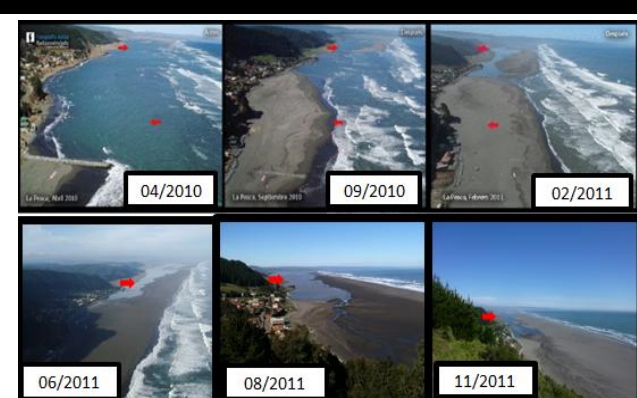
Figure 2. Recovery process of Mataquito River mouth after Chilean Tsunami of 2010. Red arrows are used to compare in time similar spatial locations on each image. (Villagran et al. , 2011)
