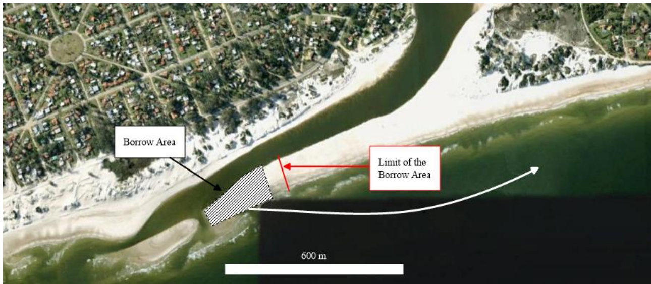
Figure 10. Outline of the borrow area proposed for La Floresta beach nourishment project.
