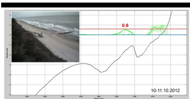
Figure 3. Output from XBeach modelling indicating breaking waves and the possibility of rip current occurrence.
