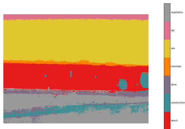
Figure 7. Infrared variance image classified using trained Conditional Random Field.
