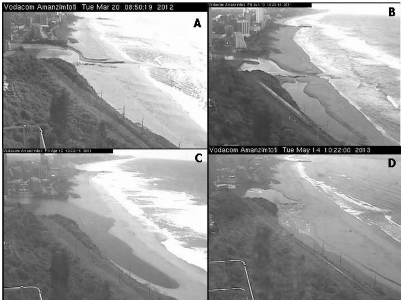
Figure 2. Amanzimtoti River and Lagoon morphodynamics. A. Baymouth bar breached after thunderstorm; B. Baymouth bar breached after thunderstorm, note that the southern outlet channel has been abandoned; C. Lagoon outlet moving to the south; D: Lagoon outlet flowing southward.
