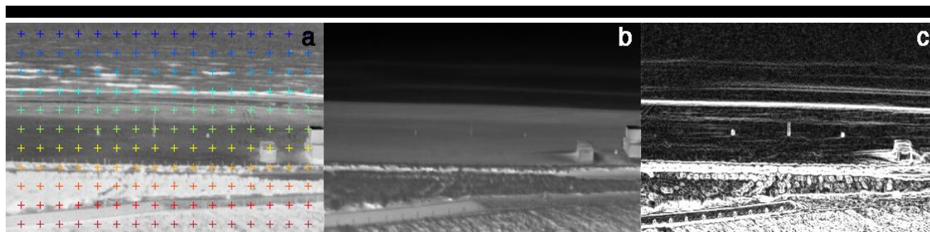
Figure 1. a) Raw infrared image. b) Arbitrary time-variance image. c) Spatial gradient in time-variance.
