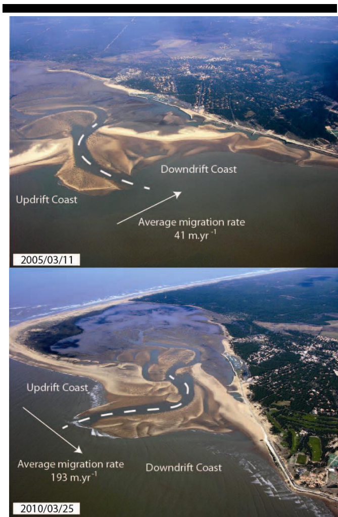
Figure 5. Oblique aerial photographs (obtained from a microlight) showing the two main orientations of the tidal inlet meander bend. Upper photo (Courtesy of Les Mattes Municipality): In 2005, the meander bend was convex in an updrift direction and counteracted the littoral drift leading to a slow downdrift migration of the tidal inlet. Lower photo (Courtesy of Les Mattes Municipality): In 2010, the meander bend was convex in a downdrift direction and the meander-induced transport was in the same direction as the longshore transport leading to a fast downdrift migration of the tidal inlet.
