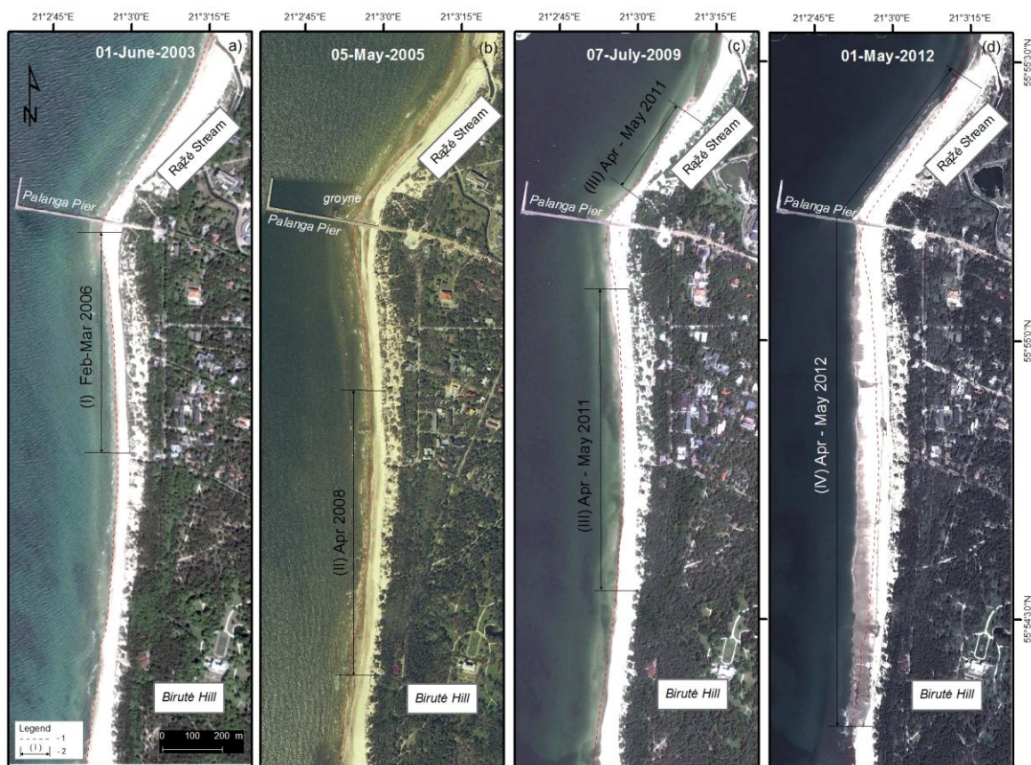
Figure 2. Documented beach nourishment sites in Lithuania and comparison of satellite images of nourished beach at different times. Numbers in legend: 1 – shoreline position in 01-06-2003, 2 – beach nourishment place, project number and date.
