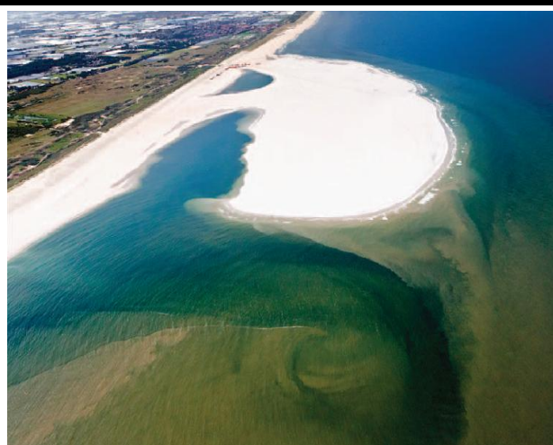
Figure 1. Aerial Photograph of the Sand Motor after completion (September 2011) looking southward showing clouds of fine-grained material. Picture courtesy of Rijkswaterstaat/Joop van Houdt.
