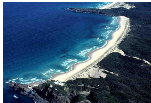
Figure 5. Rip channels and transverse bars with a rhythmic shoreline under low wave condition. Courtesy of Gallop et al. (2011).
