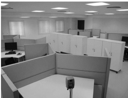
Fig. 2. Top: The layout of the office laboratory. The four speech loudspeakers are shown at the corner desks. Bottom: A photograph of the desk area showing one of the loudspeakers.
