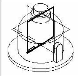
Draw the profile shown. Notice the connect relationships between the top right and bottom left corners of the rectangle and the outer line of the revolved protrusion.
