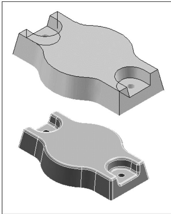
9. Thin wall the model, specifying a wall thickness of 4 mm. Leave the bottom face of the model open. To view the thin wall result more clearly, the model shown in the illustration has been rotated 180-degrees.
