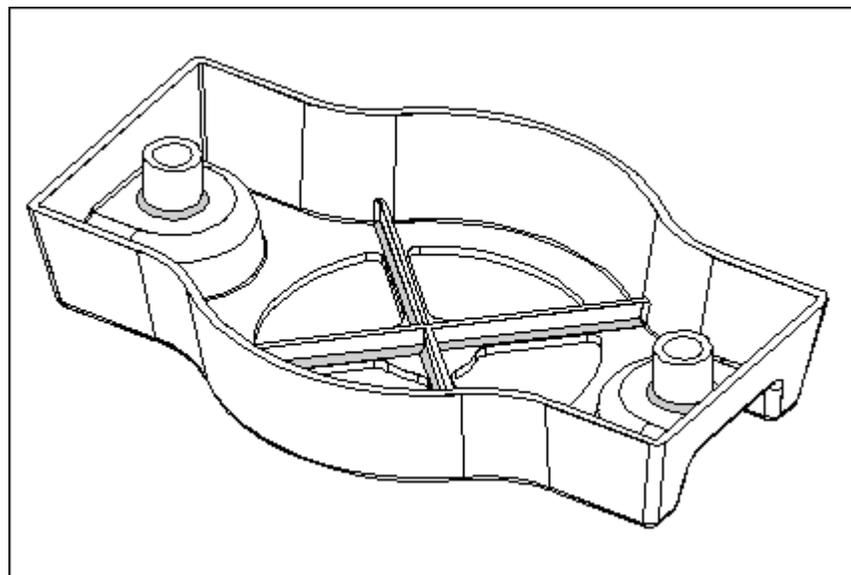
15. Add a 2 mm square groove to the perimeter of the model's bottom and a 2 mm lip to the bosses. Use the Lip command for this.
