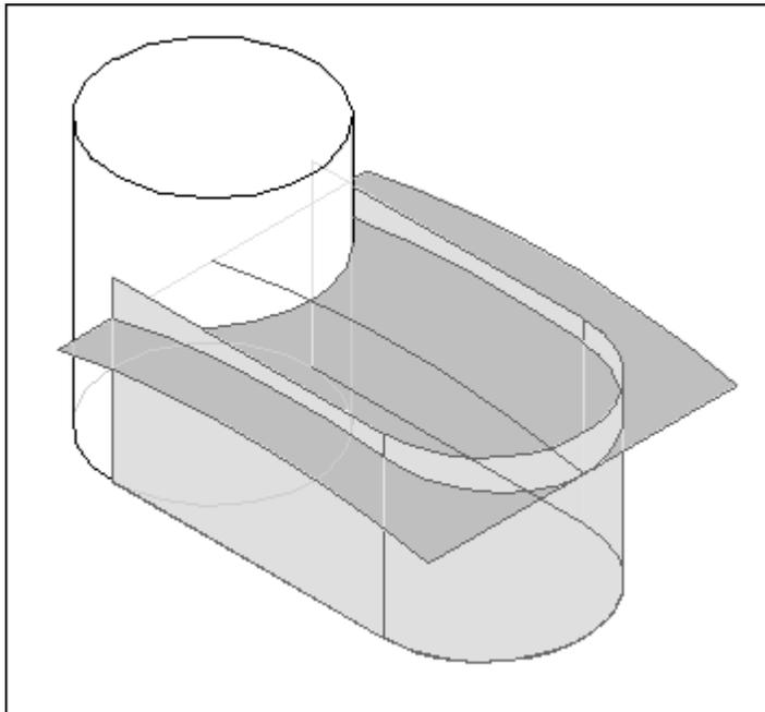
3. You will now create an intersection curve between the two construction surfaces.
