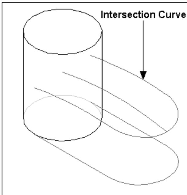
4. You will now create a swept protrusion using the intersection curve as the path curve.
