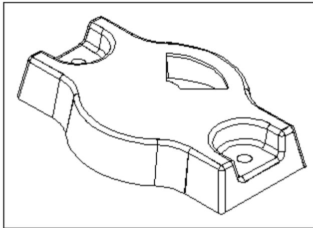
11. Add a 5 mm radius round to the four thickness edges created by the cutout you constructed in the previous step.
