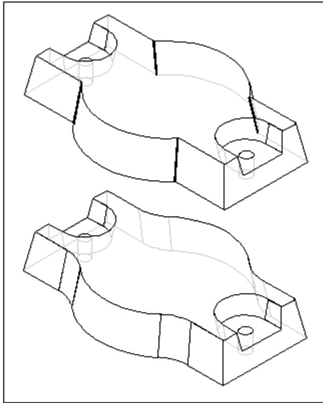
8. Add a 5 mm round to all edges shown in the illustration. Do not select hole edges nor edges around the perimeter of the bottom face.
