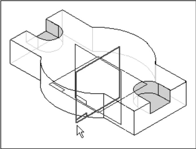
5. Add a 10-degree draft to the model. Use the bottom face of the model as the drafting plane, and draft inward from all sides perpendicular to the bottom of the model, including the sides created from the cutouts.
