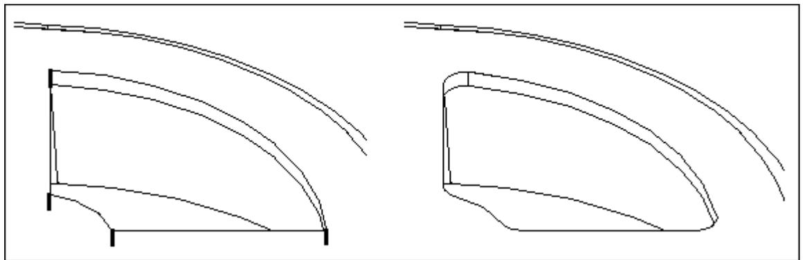
12. Create a circular pattern using the cutout and the rounds you created in the previous two steps. The pattern should have four evenly spaced instances as shown in the illustration.
