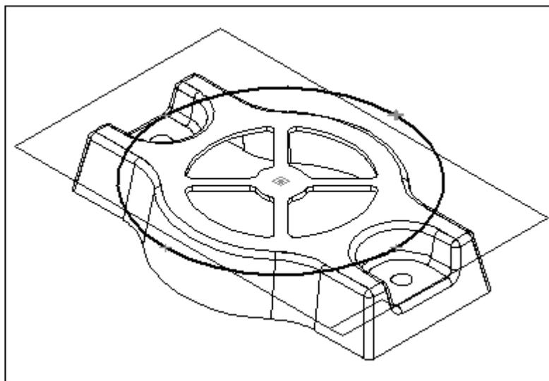
13. Construct reinforcement ribs as shown. Use the Web Network command with a parallel reference plane 10 mm off the face shown in gray. Make the ribs 3 mm thick.
