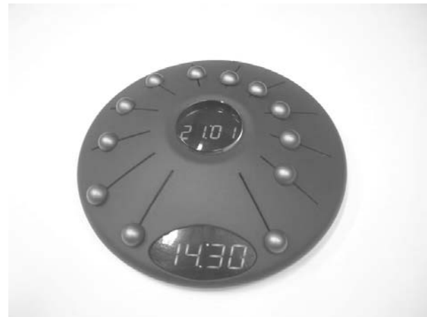
Figure. 4 The working prototype. The user can set the time by sliding the knobs towards the central alarm display. And he can do this in many different ways, eliciting him to express his mood.
