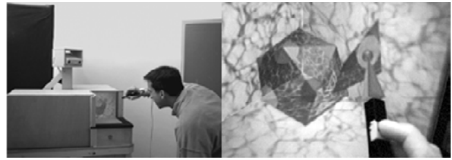
Figure 2 The head movements of the person are recorded. A computer generates 3 images, corresponding with the person's viewpoint, and projects them on 3 orthogonal screens (left). The person sees a 3D object and has a hybrid instrument with which he can interact with this object (right).
