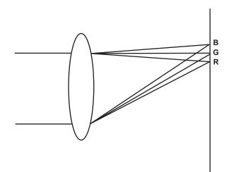
"Chromatic aberration" here refers to zoom factor chromatic aberration. Zoom factor chromatic aberration occurs since the diffraction ratio of a lens differs according to red (R)/green (G)/blue (B). Chromatic aberration on the lens itself is compensated for, but still remains in the periphery, in particular. Also, this chromatic aberration occurs on zoom lens due to a complex relationship between zoom ratio, iris and focal distance. In image terms, this is registration error.
