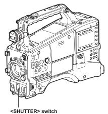
**1** Press the <SHUTTER> switch positioned at <OFF> towards the <ON> side.
