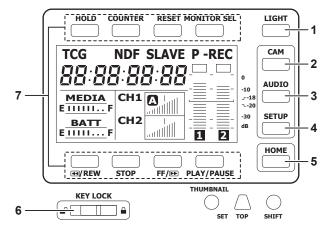
When the camera is turned on, the [HOME] screen is displayed. The status of the [HOME] screen at previous start-up is retained. 1 <LIGHT> button
