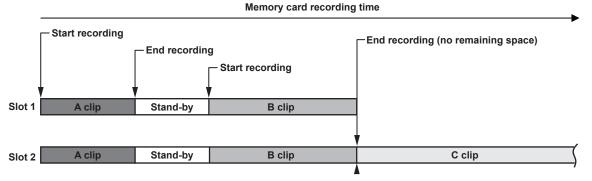
Selecting [ON] in the main menu → [RECORDING SETUP] → [SIMUL REC] will set the camera to simultaneous recording mode.
