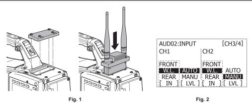
1 Remove the cover to insert the wireless microphone receiver and secure it with the screws. (Fig. 1)
