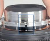
6. Tighten the eight torx screws with the T6 torque wrench using a torque of 0.25 Nm.
