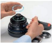
12. Place the black EF adapter ring on the lens barrel and tighten the screws using a torque of 0.25 Nm.
