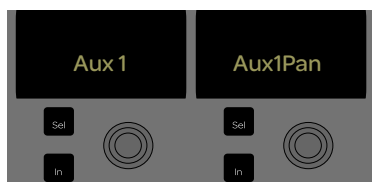
Aux send level controls (left) and send pan (right)
