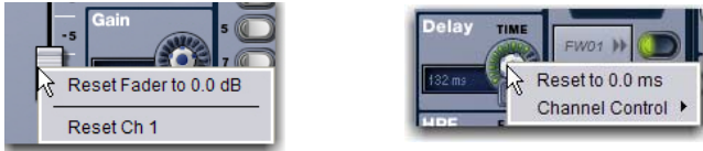
Right-clicking channel strip controls on-screen
