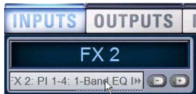
Jumping to a plug-in on an FX Return
