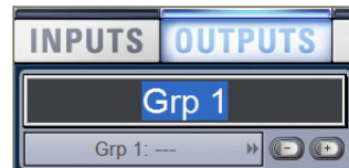
Changing the name of an Output channel on the Outputs page
