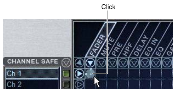
Enabling recall safe for channel 1 fader
