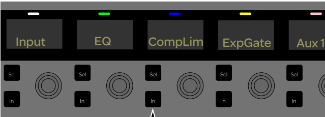
Channel Control encoder In switch
