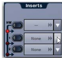
Click to assign (left); click to go to the plug-in rack (right)
