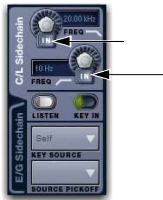
Key HF button (top) and Key LF button (bottom)
