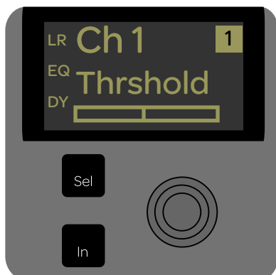
Comp/Lim Threshold assigned to channel encoders
