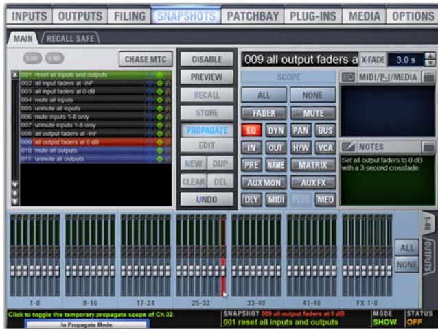
Propagating an EQ change for a channel
