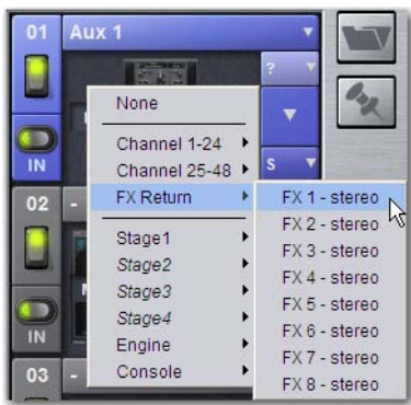
Assigning plug-in output to an FX Return
