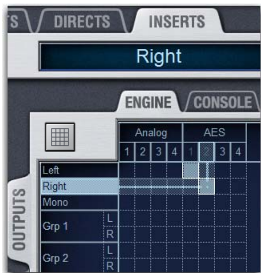
Assigning a hardware insert on the Inserts tab of the Patchbay
