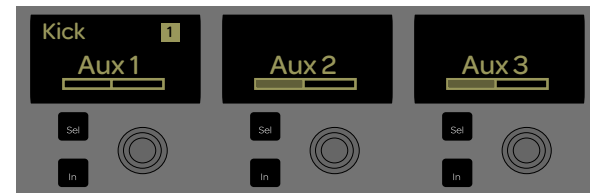
Channel Control with Auxes 1–8 assigned to Channel Control (Aux sends 1–3 shown)
