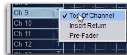
Selecting a Direct Output pickoff point in the Patchbay
