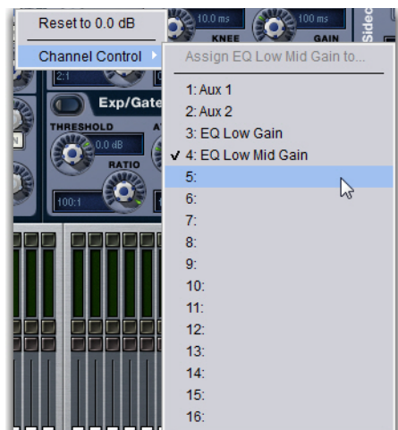
Assigning a parameter to Channel Control on-screen
