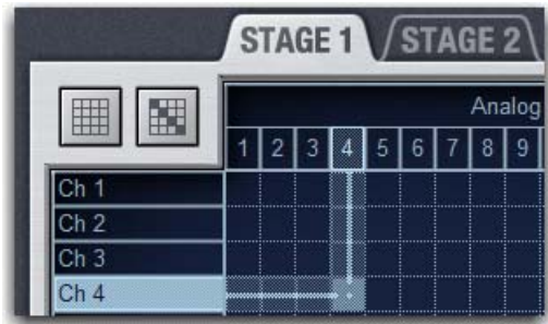
Assigning input sources in the Patchbay
