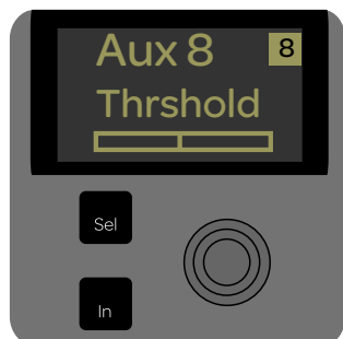
Comp/Lim Threshold assigned to a channel encoder
