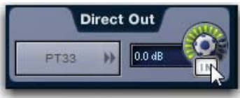
Activating a Direct Output on the Directs tab of the Patchbay
