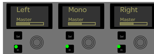
Main busses assigned to the Global Control encoders
