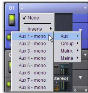
Assigning plug-in Input source to an Aux bus
