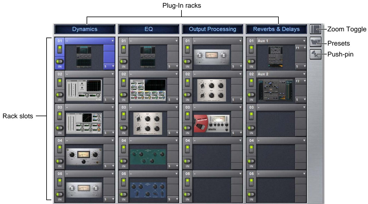
Figure 2. Plug-In racks and rack slots, Main view, with custom rack names shown.
