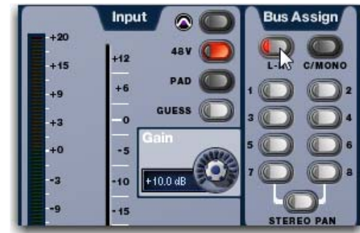
Assigning an input to the Mains Left-Right bus
