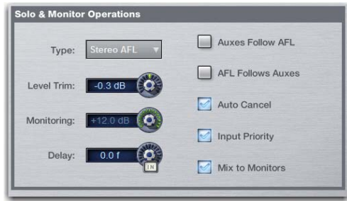
Solo controls on the Options > Busses tab
