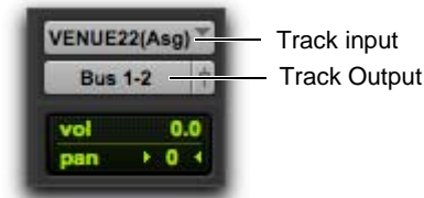
I/O assignments for Assignable outputs from S3L
