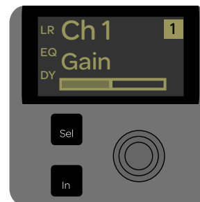
Gain assigned to the channel encoders
