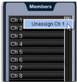
Removing an input assignments from a bus
