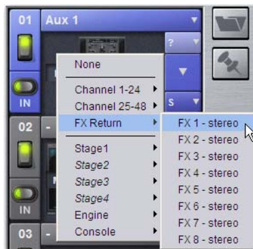
Assigning plug-in output to an FX Return
