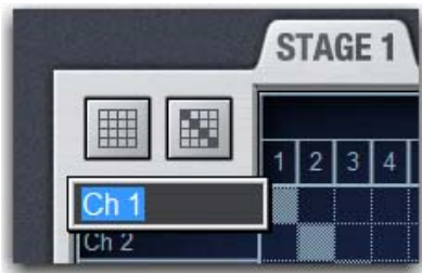
Naming and Input Channel from the Patchbay
