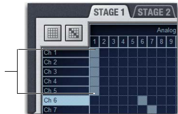
A hardware input routed to multiple Input Channels
