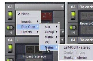
Assigning monitor output to a bus-fed plug-in
