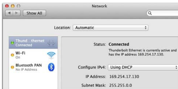
Mac Network Settings screen showing an active network connection to the S3L system
