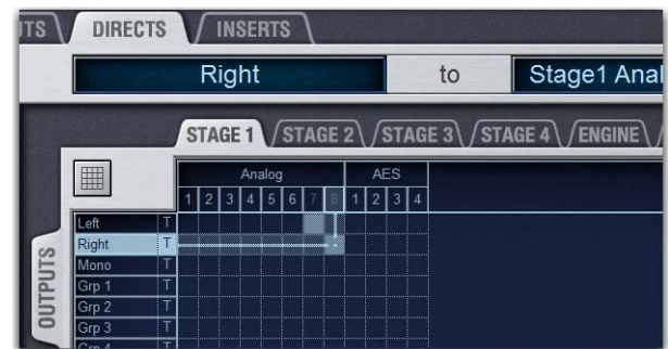
Assigning a Direct Output in the Patchbay
