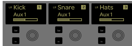
Channel encoders with Aux 1 sends assigned
