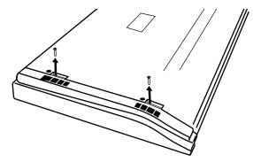
Removing screws from the bottom panel
