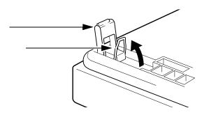
The two larger, detached riser brackets elevate and angle the unit more than the foldout legs. Use moderate force to snap them into the bottom panel.
