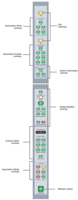
Figure 2. Global Controls section
