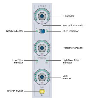
Low Filter and High-Pass Filter controls in the EQ section
