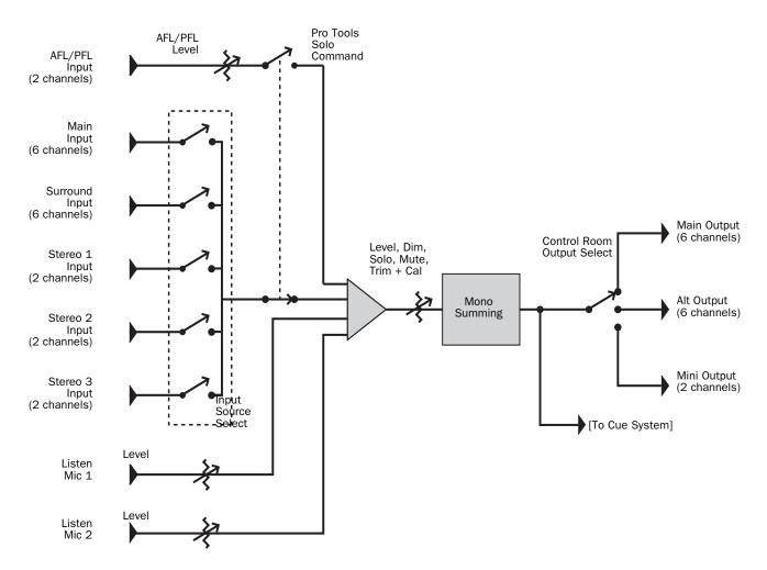
Figure 7. Control room monitoring system block diagram
