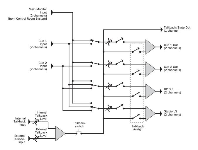
Figure 8. Headphone/Cue system block diagram
