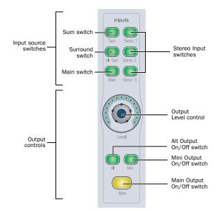
Input source switches and Output controls
