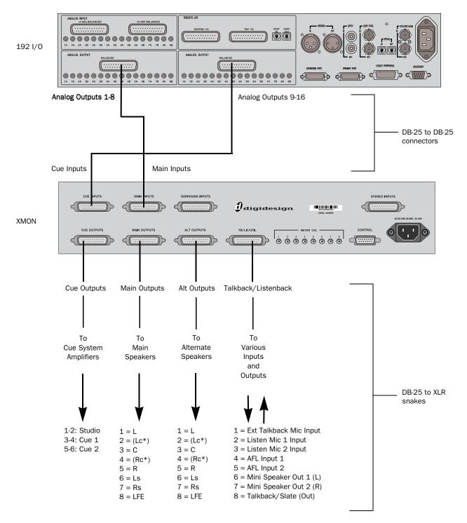
\* Main Speaker Outputs 2 and 4 are active on XMON, but Lc and Rc outputs cannot be controlled independently from the D-Command monitor section. Global Volume, Solo, and Mute controls affect all outputs.
