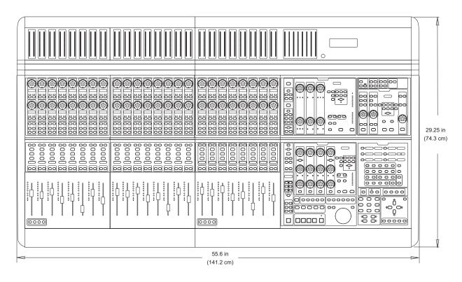
D-Command top dimensions (Main Unit and Fader Module)
