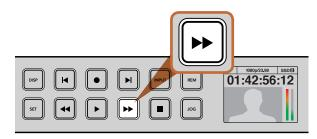
The fast forward button on the front of HyperDeck Studio models lights up when fast forwarding through clips.
