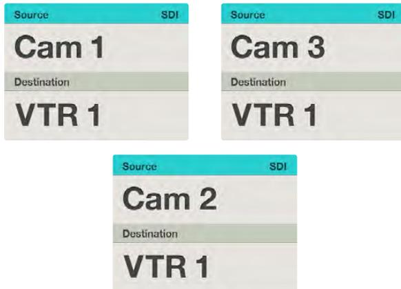
In this example, a customized Cam button has been selected so only cameras will be listed as sources, on the LCD, when the scroll wheel is rotated. This provides a fast way to find a video source because you only have to scroll through a short list of equipment.
