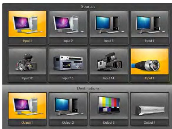
Pushbutton views provide an intuitive, icon-driven representation of the Videohub connections
