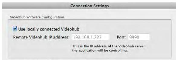
Select the "Use locally connected Videohub" checkbox on a Videohub Server computer.
