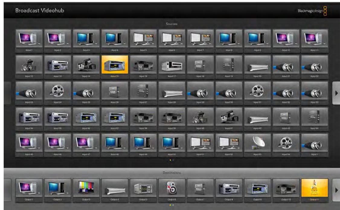
Each Pushbutton view is divided into an upper panel of buttons representing video sources, and a lower panel of buttons representing video destinations.
