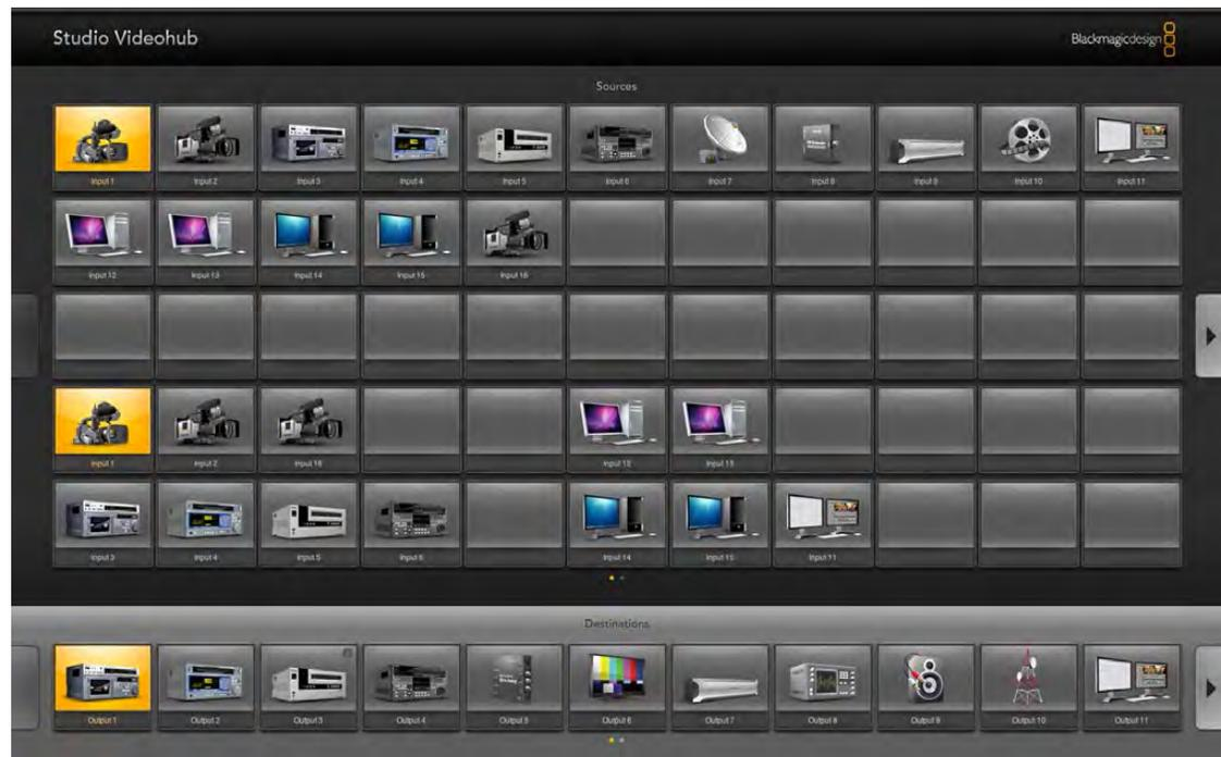
Full Screen 24" Pushbutton view showing an example of duplication and grouping of inputs. Two, illuminated instances of Input 1 can be seen in this example. Grouping of inputs can enable quick identification and location of video sources of the same type, e.g. all available cameras.
