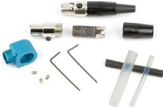
Adapter kit to build either a 3-pin or 5-pin TA Series right angle connector. Includes standard 5-pin connector, modified 3-pin insert and backshell, aluminum right angle housing, strain relief tubing, set screws and wrenches.
