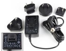
AC power supply for IGBT4 transmitters; 100-240 V, 50/60 Hz, 0.3 A input, 12 VDC regulated output; 7-foot cord with LZR threaded locking plug and interchangeable blades/posts for use in Europe, UK, Australia and USA (sold separately).
