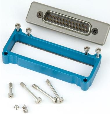
Adapter kit for Unislot® camera slots such as those provided on Ikegami® and Panasonic® cameras.\* Includes bezel, hardware and rear panel DB25 connector wired for power and audio connections.
