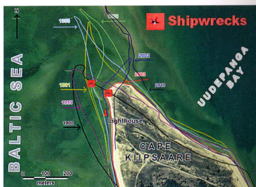
■ Figure 4.6 Shoreline changes during the period from 1900–2010 (shipwrecks found in 2000 and 2010 are also indicated). Key: black = 1900; Purple = 1955; Yellow = 1981; Green = 1988; Lilac = 1998; Light blue = 2002; Red = 2008; Dark blue = 2010
